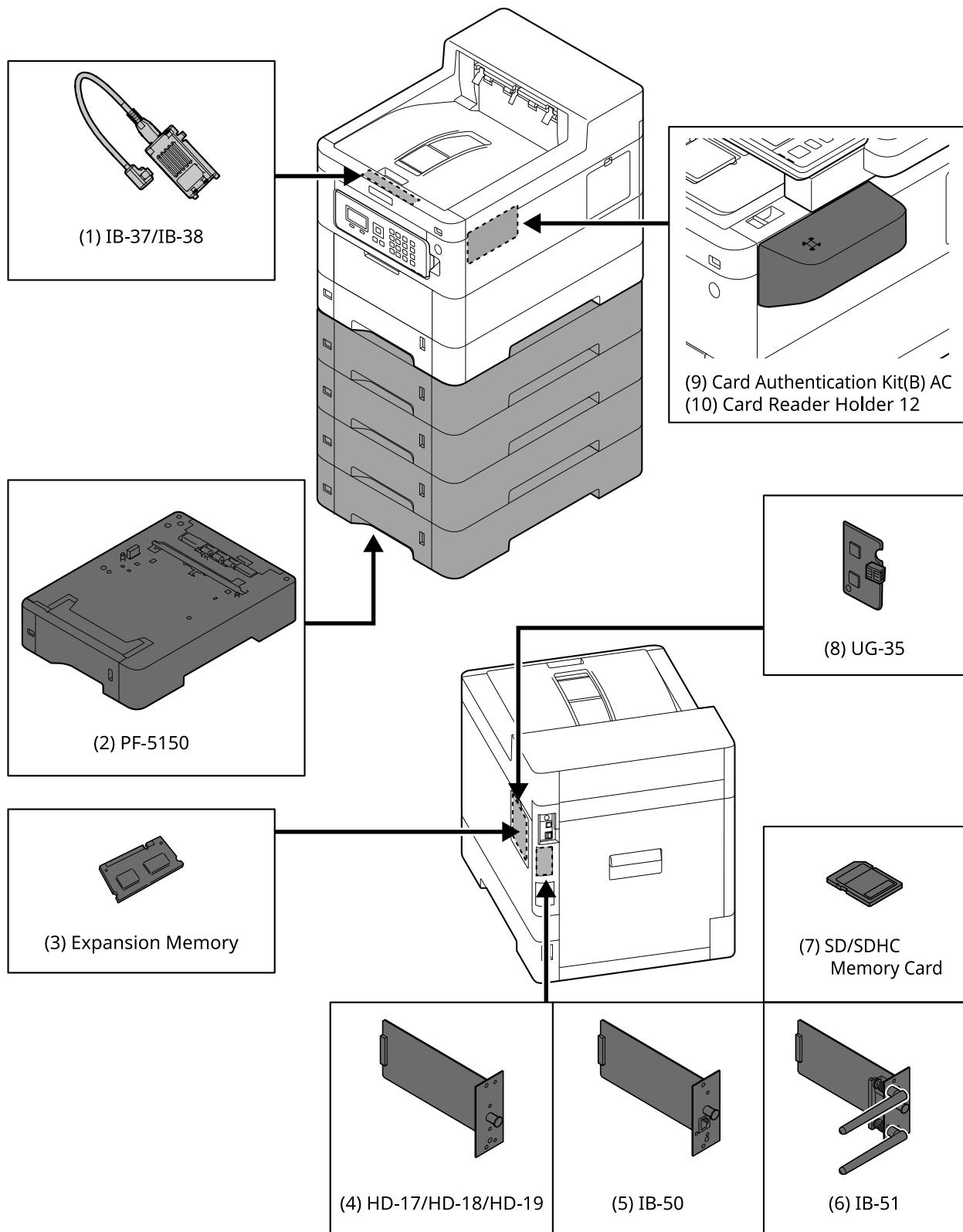
**1 IB-37/IB-38 <Wireless network interface (USB: 5GHz/2.4GHz)>**
